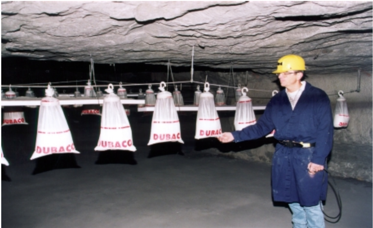
Figure 5.2.3a: Distributed barrier layout in B-drift
