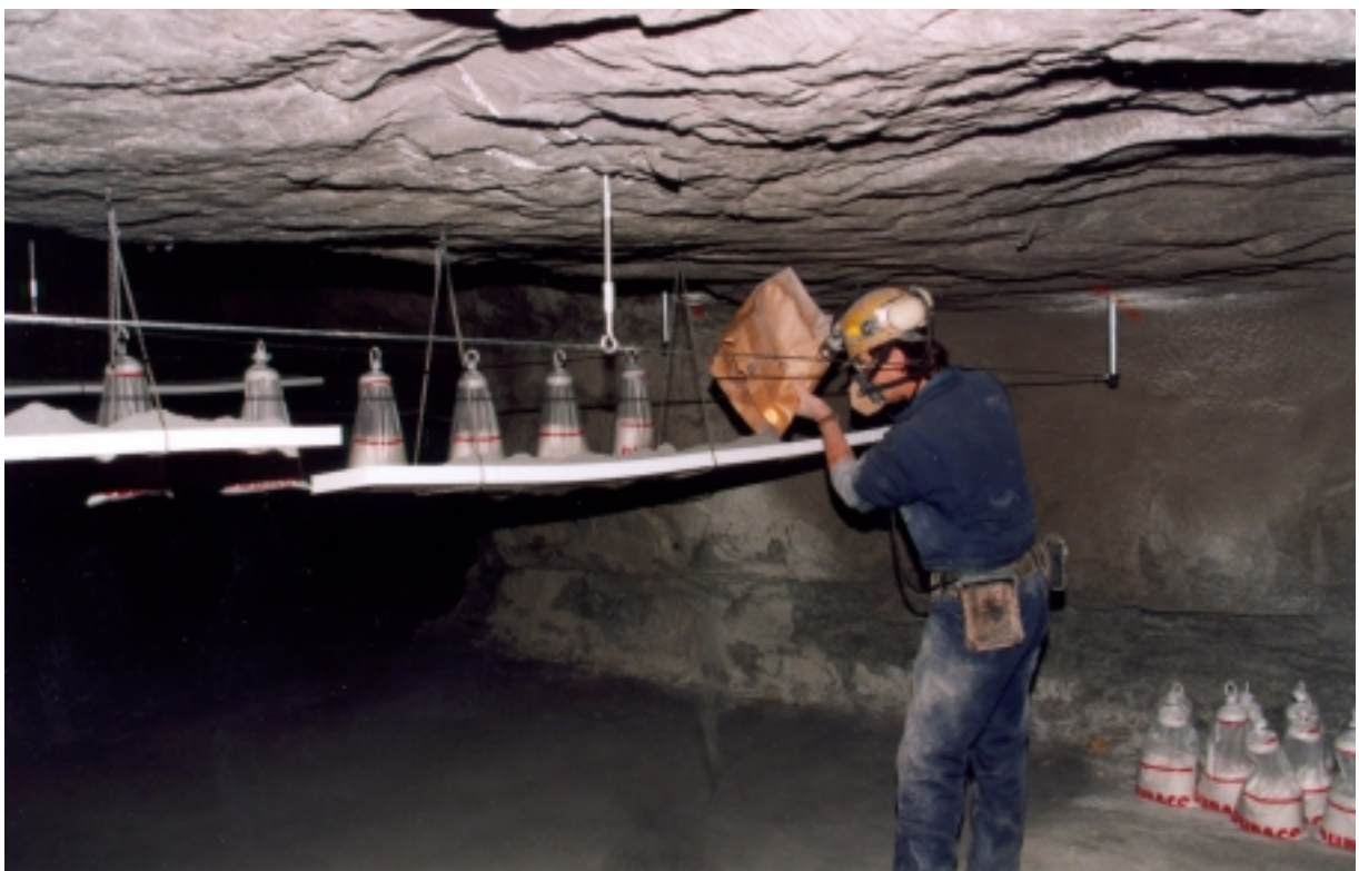
Figure 5.2.1b: Photograph showing coal dust distribution on shelves
