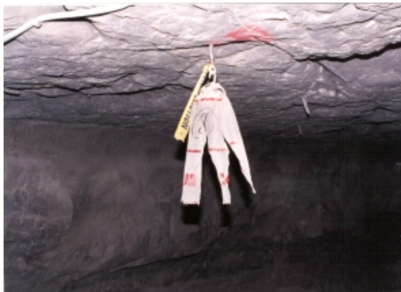
Figure 5.3.1.3b: Post-explosion photograph of an emptied bag
